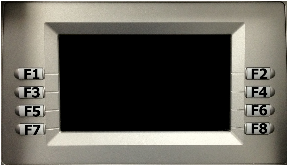
G2500 LCD display Function Key layout
